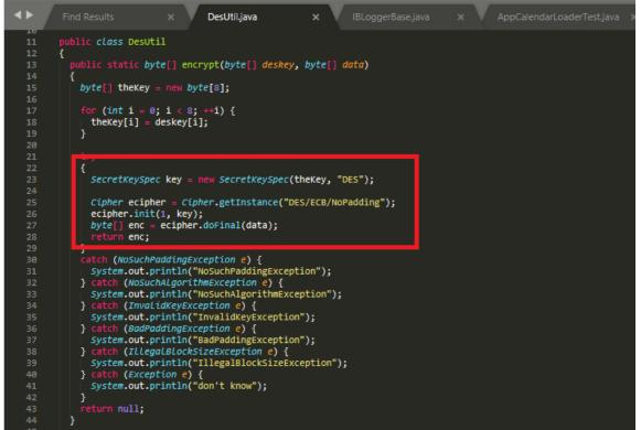
Figure 1: The screenshot shows the encryption using unsupported algorithms ("DES/ECB/NoPadding") in DesUtil.java on line 25
